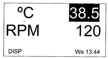
3. Turn or spin the Knob to reset the setpoint (in this example, turn the Knob left to decrease the setpoint to 37.0).
