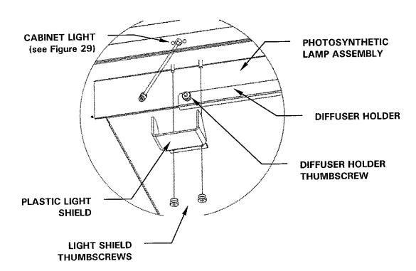
Figure 30: Replacing Photosynthetic Lamps
