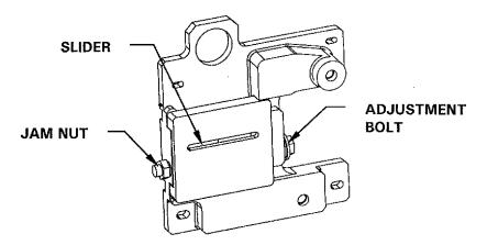
To adjust door tension, you will need two 9/16-inch open-ended wrenches and two wood blocks, each approximately 3/4 inch x 1½ inches x 6 inches, to protect the door gasket from the upper door arms during this procedure:
