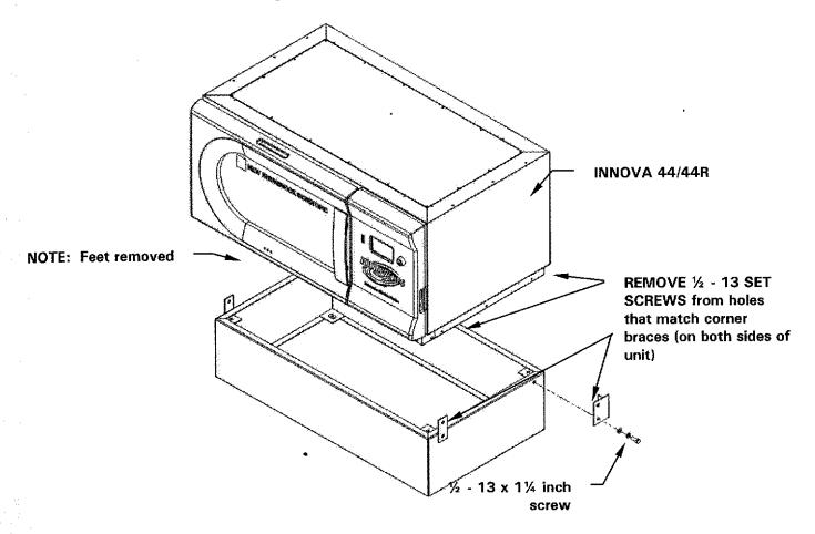
Figure 3: Mounting Shaker on Base
