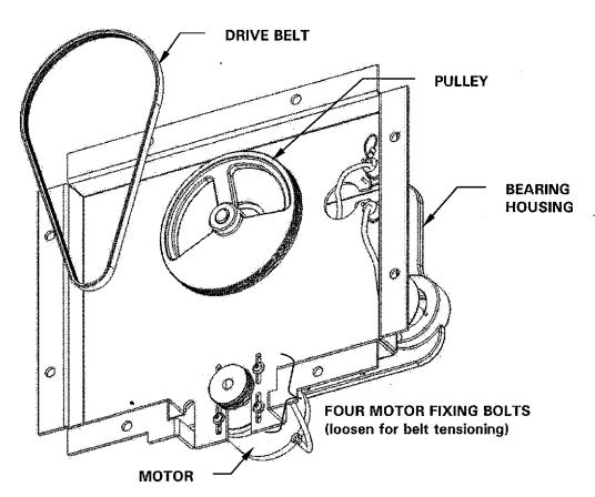
Figure 35: Belt Replacement & Adjustment
