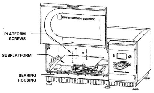
Figure 10a: Installing Subplatform
