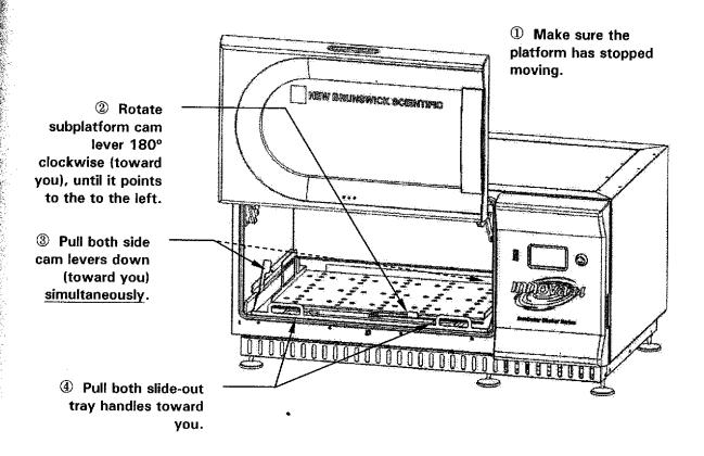
Figure 27: Disengaging Slide-Out Platform
