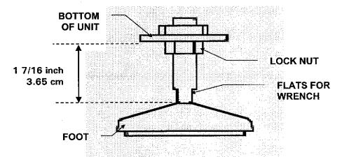
Figure 2a: Adjustable Foot (as shipped)
