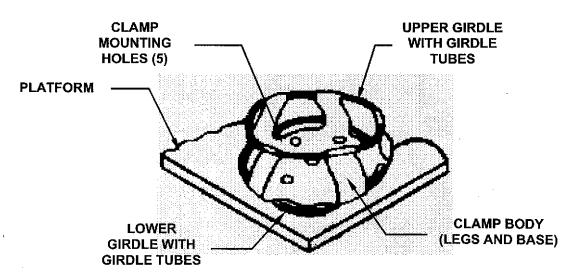
Figure 11a: Double Girdle Clamp Installation
